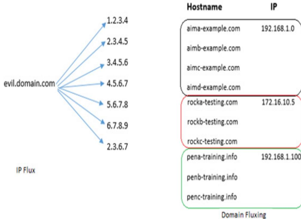
Figure 2: An example of IP-Flux and Domain-Flux
